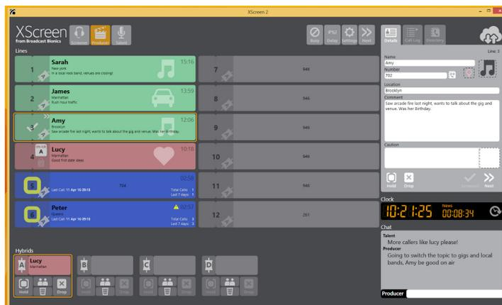
XScreen software comes with every Hx6 Engine purchase and provides call control, call screening, data capture, and chat functionality enabling you to quickly answer, screen, and route calls using multiple PC clients. The cloud-based database keeps a log of calls and provides further alert and directory functionality.
