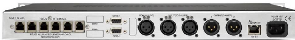
Around back, you'll find audio I/O, GPIO, and Telco connections. Hx6 connects directly to 6 POTS lines. Separate analog or optional AES digital I/O is provided for each hybrid, as well as a Program-On-Hold input, GPIO connections for speaker muting, ring tallies, et cetera.
