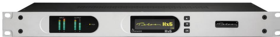
Like all Telos talkshow systems, the Hx6 front panel is simple and informative, with separate send and receive meters for each hybrid, a Program-On-Hold audio presence indicator, a high-resolution OLED display for setup, and navigation keys for quick adjustments.
